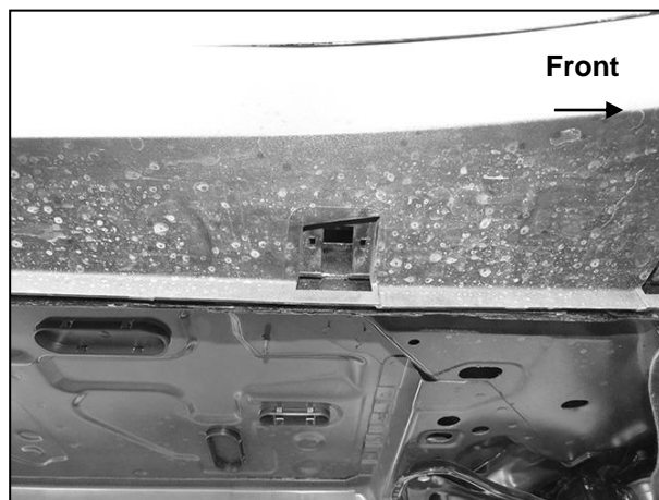
(Fig 2) Passenger/right #2 clip removed
