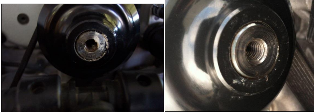
Figure 26: OEM Drive Pulley | Left: Untampered | Right: Tampered With
