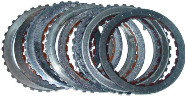
Figure 10A: Damaged Clutch Discs
