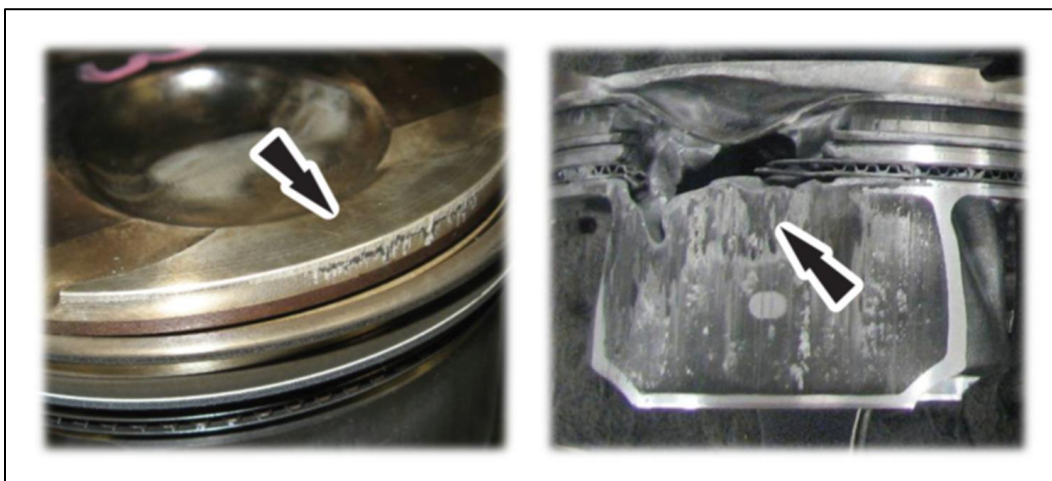
Figure 4: Light/Heavy Knock Damage
