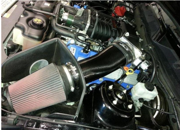
Figure 27: GT500 Aftermarket Air Filter, Inlet Tube, Throttle Body & Supercharger
