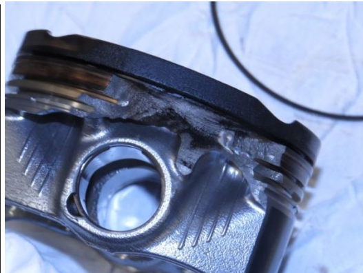
Figure 3: Piston Ring Land Damage
