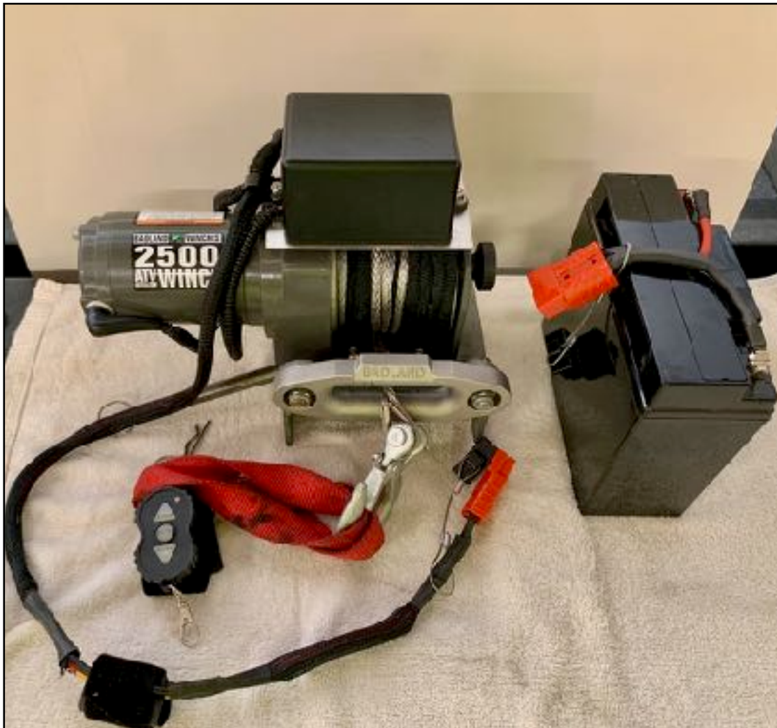
Winch on base, with wiring, wheelchair battery and wireless remote.
