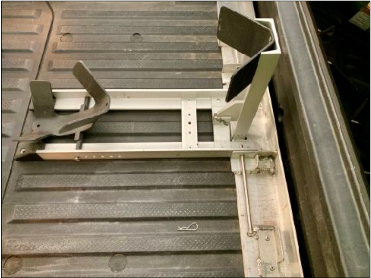
Folding Condor wheel chock and mounting rail, Chock mounts with one pin. 2017 Ridgeline version.
