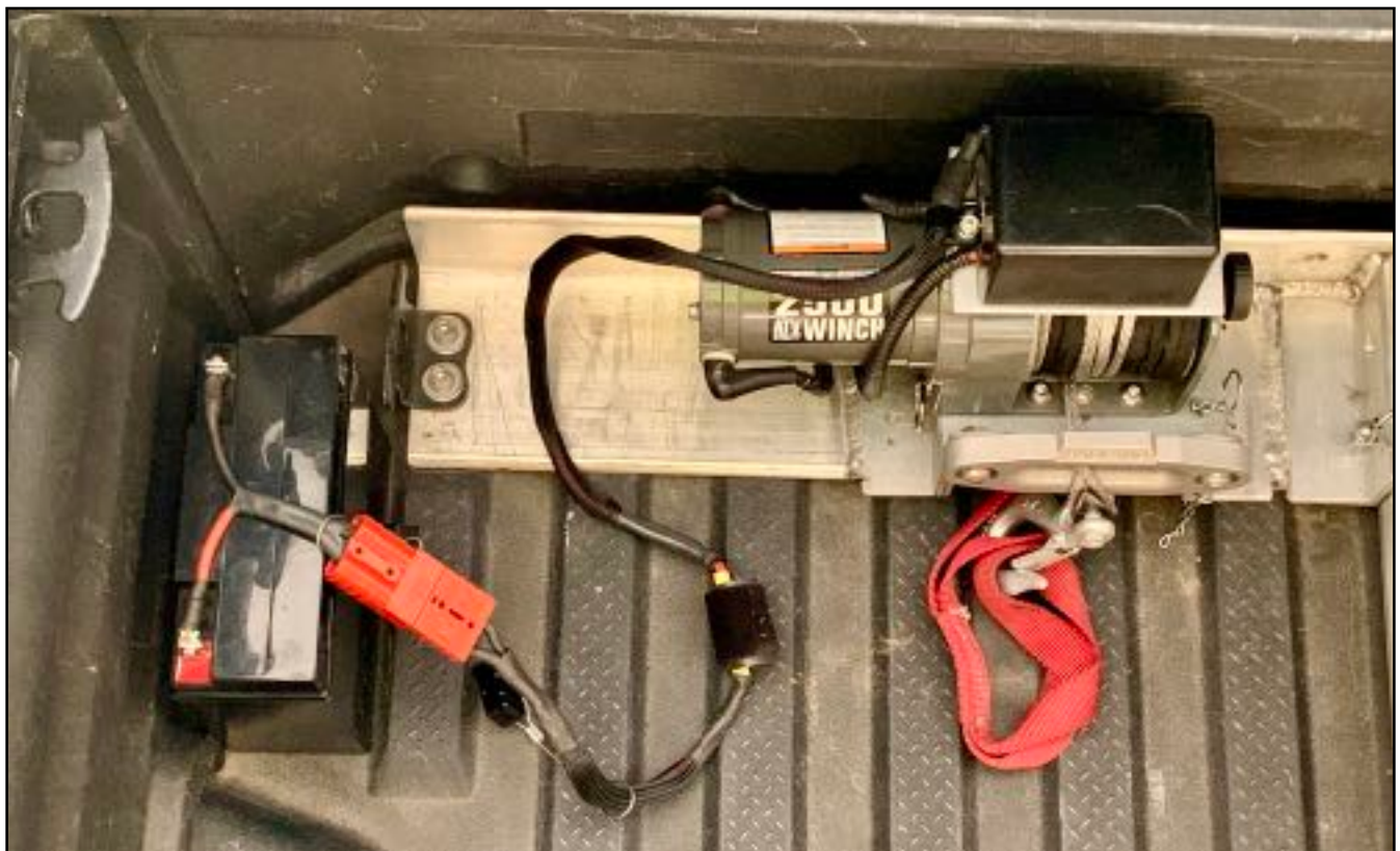
One pin mounted Winch, battery, and wiring. 2017 Ridgeline version.
