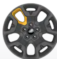
17" machined-face Dark Tarnish-painted aluminum with Tremor Orange-painted pocket Included on Tremor Off-Road (17V) and Tremor Appearance Package (17C)
